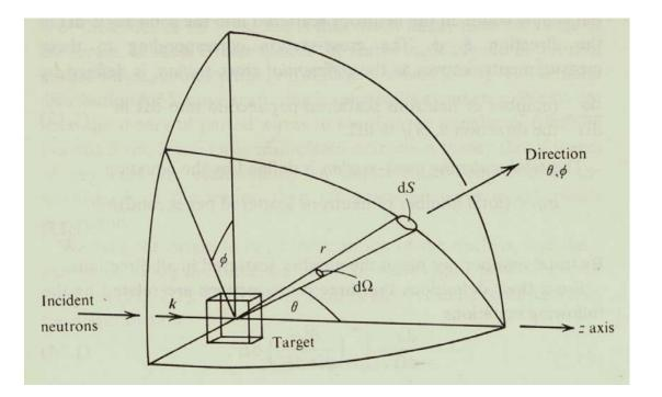
$\Phi = \text{number of incident neutrons per cm}^2 \text{ per second}$   $\sigma = \text{total number of neutrons scattered per second / } \Phi$   $\frac{d\sigma}{d\Omega} = \frac{\text{number of neutrons scattered per second into } d\Omega}{\Phi \, d\Omega}$   $\frac{d^2\sigma}{d\Omega dE} = \frac{\text{number of neutrons scattered per second into } d\Omega \& dE}{\Phi \, d\Omega \, dE}$
