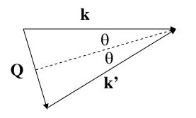
Neutron diffraction measures the differential scattering cross section  $d\sigma/d\Omega$  as a function of the scattering wavevector (**Q**)
