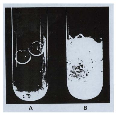
Both tubes contain borosilicate beads + pyrex fibers + solvent. (A) solvent refractive index matched to pyrex;. (B) solvent index different from both beads and fibers – scattering from fibers dominates
